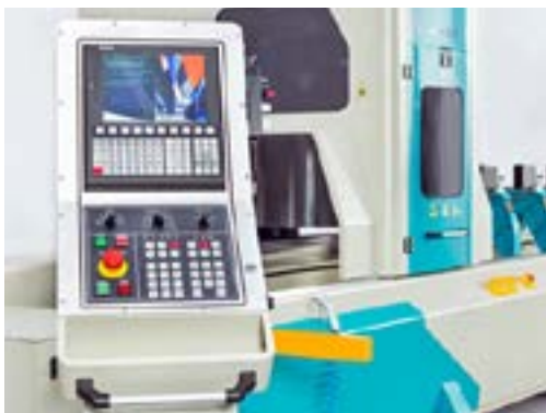
Movable control panel
