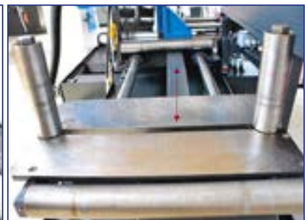
Feed gripper 500 mm reversing and switchable as pusher gripper
