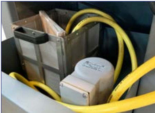
Lateral coolant system with pump on castors
