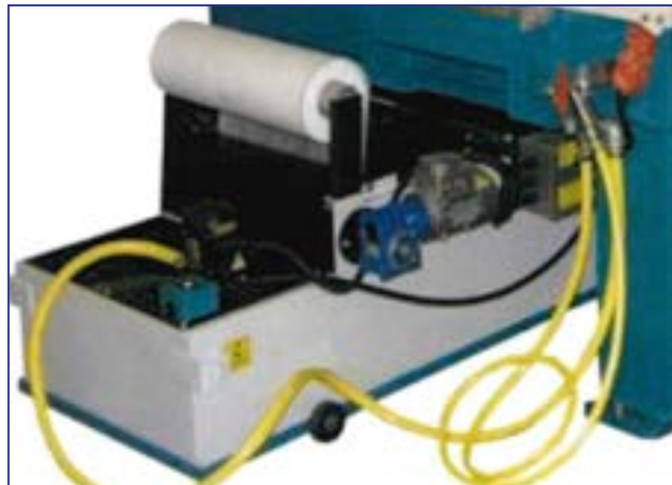
Option with paper band filter instead of tray on castors with removable screen
