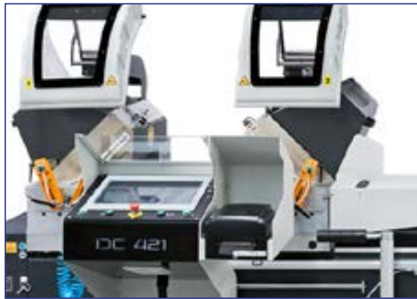
Mobile control panel
