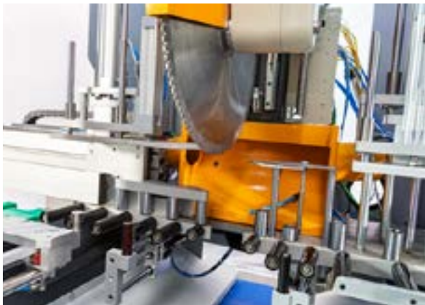
Vertical saw cut
